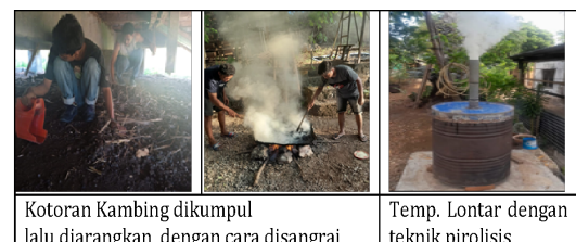
Gambar 3. Proses Karbonasi Material Biomassa
